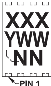
8-Lead DFN (2x3x0.9 mm)
